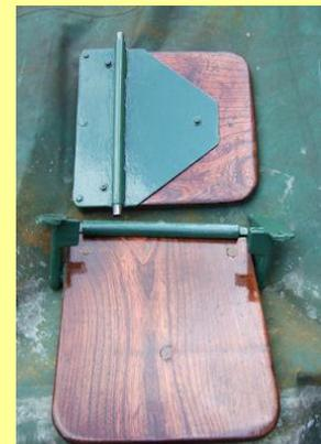
Cab seats now restored - to the standard we want for 1014 herself. The seats will be fitted on to the cab side sheets.
