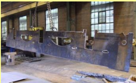
03/12/2011 - newly cut tender mainframe at Multi-Tech. Although the plate is marginally thicker (0.026 in / 0.65 mm) than original, the cutting tolerance achieved was within 1.5 mm over the full length, which is exceptional.
