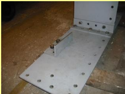
26/02/2011 - brake trunion brackets fitted to new 'A' frame.
