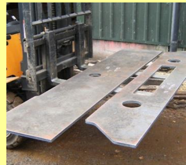
03/12/2011 - newly cut front and rear buffing plates for new tender frames.
