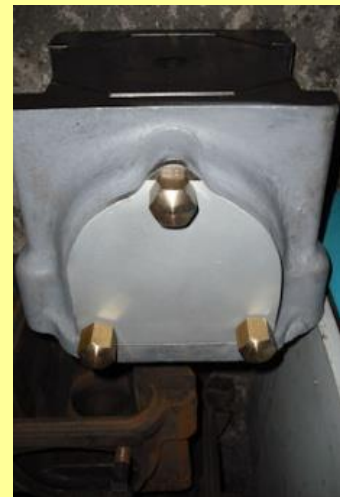
09/10/2010 - Axlebox in workshop grey, fitted with an axlebox cover bolted to the axlebox with some of the domed axlebox cover bolts produced for the task.
