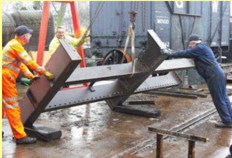
26/02/2011 - Turning the tender ladder frame over
