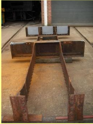
26/03/2011 - ladder frame almost complete - riveting new 'A' frame is the biggest task to undertake. Considering having frame sandblasted to remove rust, but its size is a problem.
