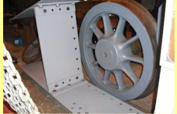
01/01/2011 - Tender 'A' frame assembled and ready for riveting.
