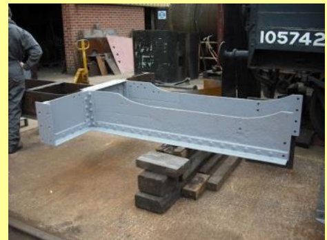
04/06/2011 - cleaned section of ladder frame primed, while work continues on the rest.
