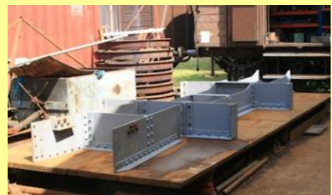
06/08/2011 - 'A' frame and ladder frame positioned on steel slab being readied for joining.
